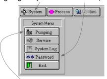
3. On the pumping page (System>Pumping) vent the load lock by clicking STOP and then VENT
