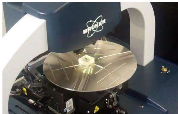
Figure 3: Sample Loaded on the Theta Sample Fixture (Chuck)
